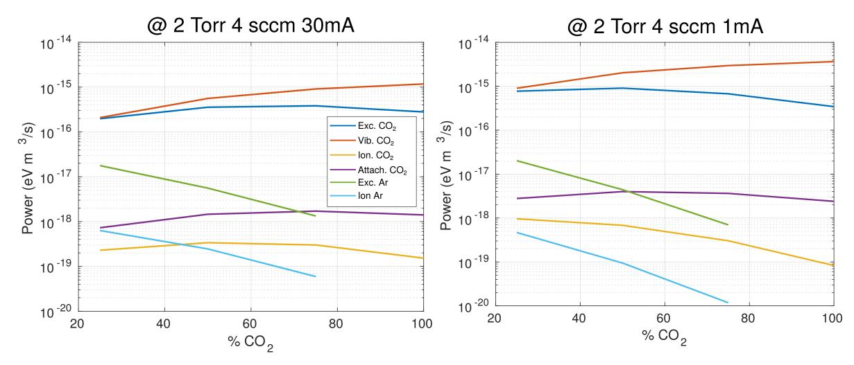
• For all working conditions the **power spent by electrons on** excitation and ionization of **Ar is negligible** when compared with the power spent on  $CO_2$ .
