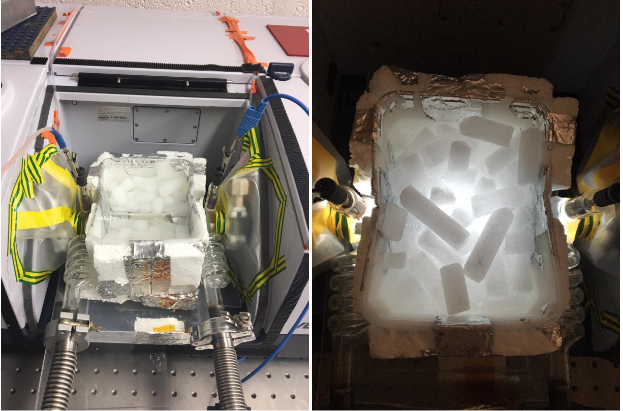
Figure 4.2: Discharge reactor immersed into a mixture of dry ice and ethanol and positioned in the sample compartment of the FTIR when the plasma is OFF (left) and ON (right).
