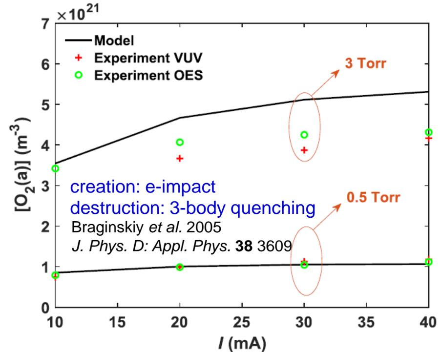
The scattering of measurements shows that model validation should focus on the **prediction of trends and orders of magnitude**
