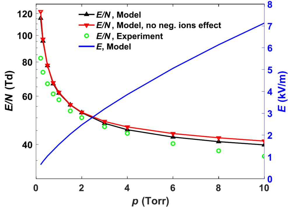
Predicting the experimental **gas temperature** and **maintenance reduced electric field** is key to model validation
